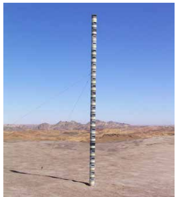
Figure 36: Multivertical dust sampler
