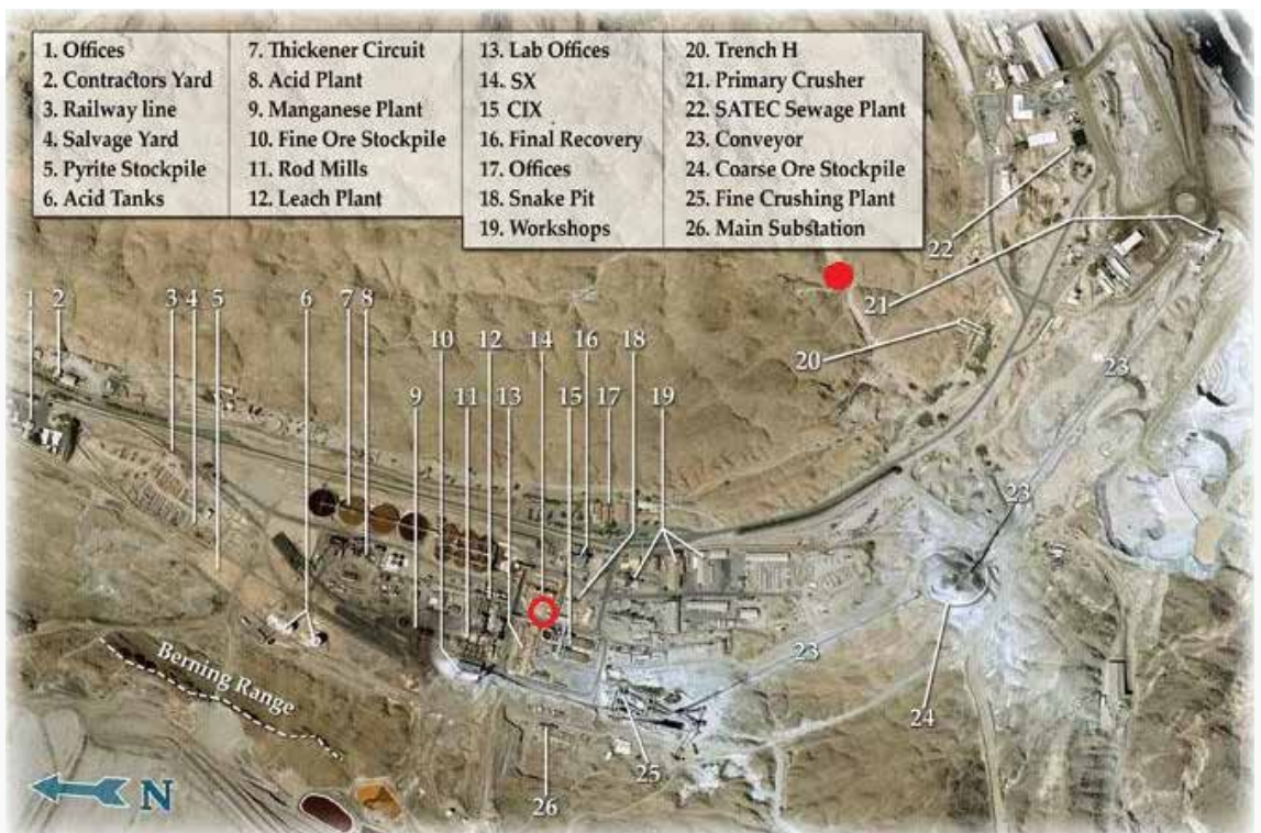
Figure 17: Plant layout showing the controlled areas: 14 – SX plant, 16 – FPR, Decontamination facility (red circle within mine site area), Radiation Source Bunker (full red circle on top of map).
